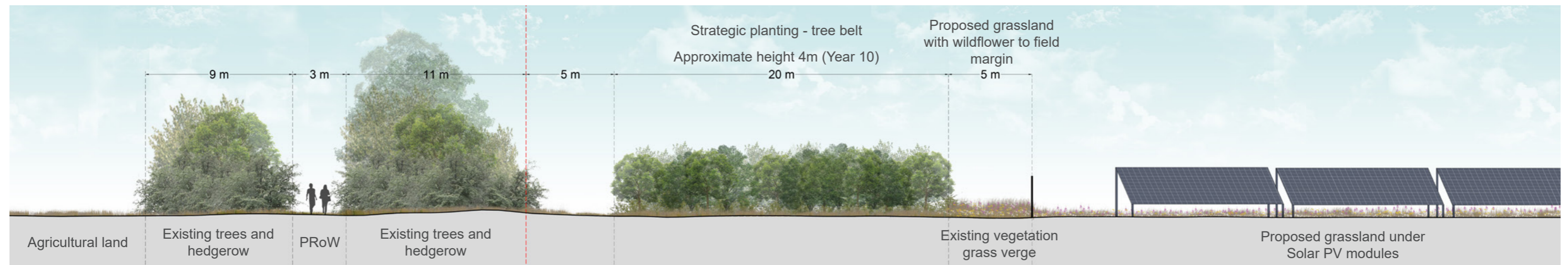
Figure 6.8: Indicative section through PRow (Ash/11/1) at Long Plantation
